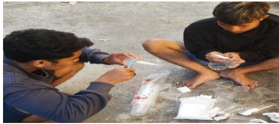
Figure 3. The process of perforating plastic cups
