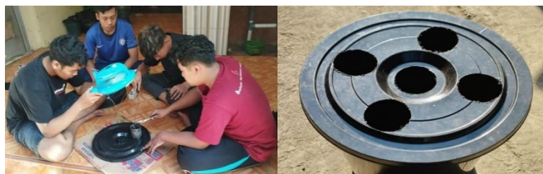
Figure 2. The process of punching the bucket lid, punching the bucket can be from 5-8 holes
